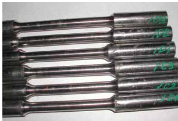
Fig. 40. Specimens for fatigue test under rotating bending load
