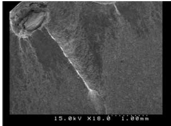
Fig. 43. Fatigue propagation area
