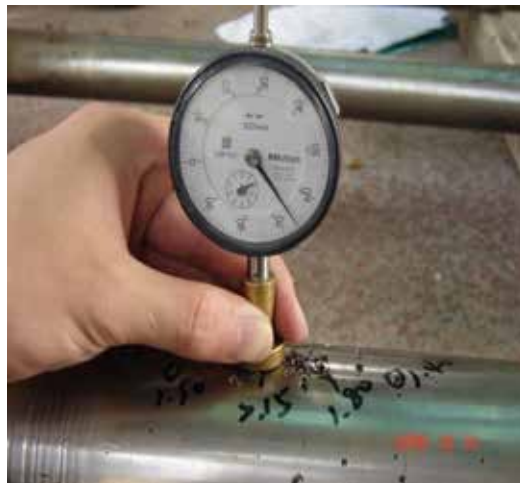
Fig. 2. Measuring depth of pitting deep
