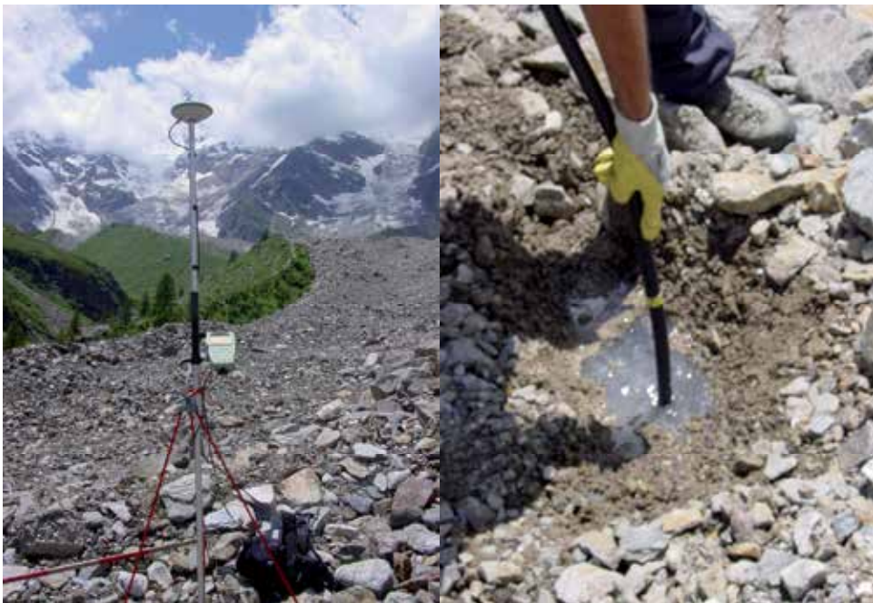
Fig. 11. Installation of an ablation stake using a stream driller and D-GPS measurement (Photo P. Federici)
