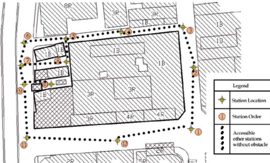
Fig. 2. Survey Planning for Scanner Station
