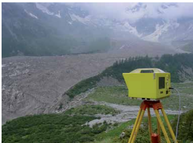
Fig. 4. The Optech ILRIS-3D laser scanner during a field measurements (photo P. Federici)
