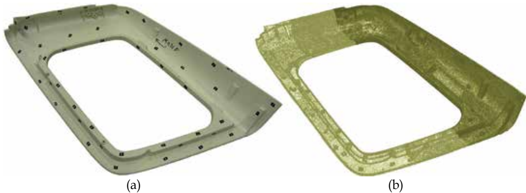
Fig. 15. (a) Physical model; (b) final polygonal model of the door chassis
