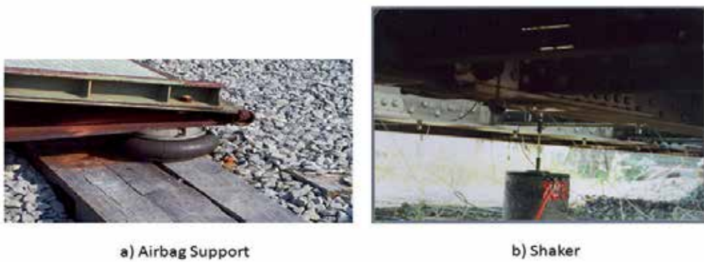
Fig. 12. Testing Setup: a) Airbag and b) Shaker
