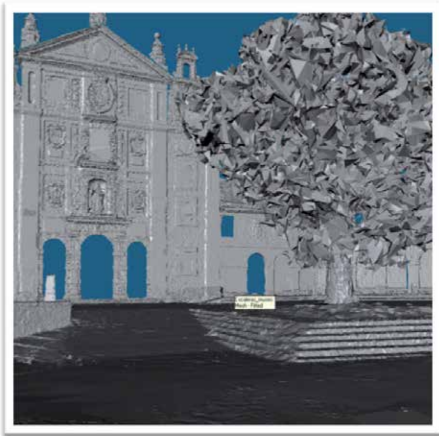
Fig. 10. Solid model of the door of the Church of the Convent of Santa Teresa.
