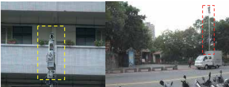
Fig. 3. The device raising 3D scanner and working on vehicle
