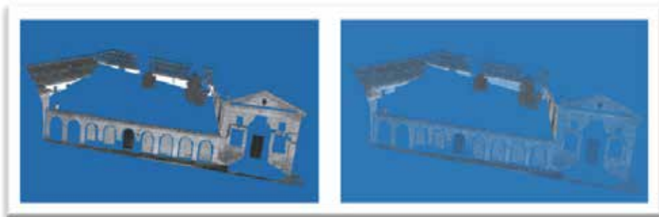
Fig. 7. General scan of the façade before and after applying a 100mm spatial sampling.
