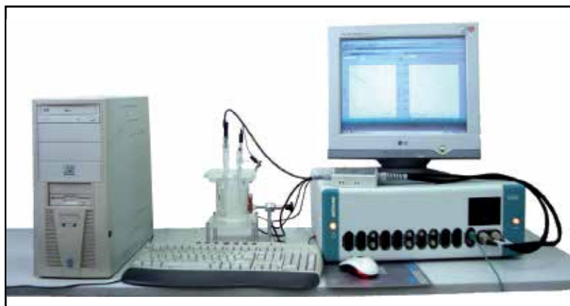
Fig. 3. The set of appliances for the electrochemical corrosion testing by EIS technique.
