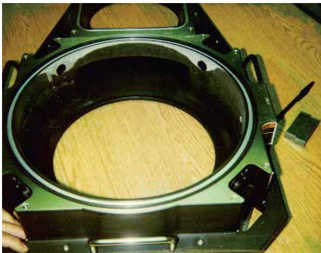
Fig. 5. Anodized aluminum is fully removed under Cl_2/BCl_3 plasma after only 1,800 wafers in production (about 60 RF hours). The special attacking pattern depends on the local plasma density and gas concentration.
