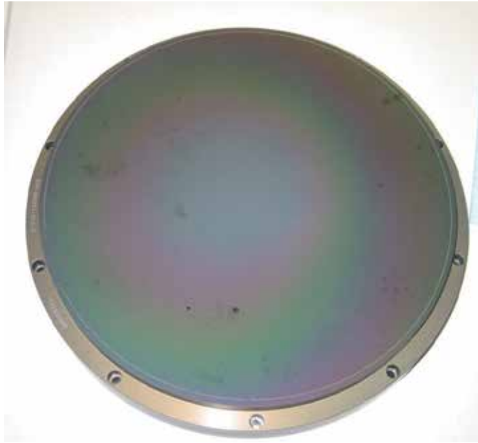
Fig. 7. A uniform AIOF film (rainbow color) covers the ceramic surface of a used electrostatic chuck after silicon etch processes.
