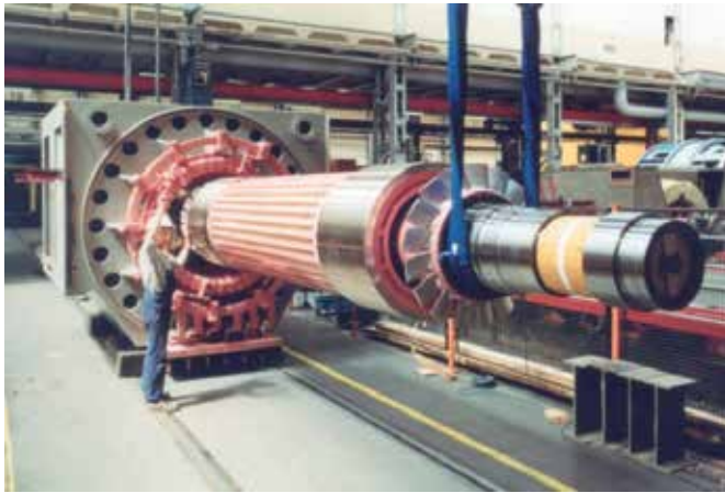
Fig. 26. Generator shaft with retaining rings, X8CrMnN 18-18 [ETE-11].
