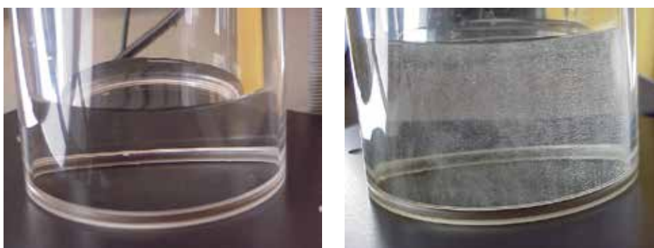
Fig. 24. Acidic corrosion resistance of two test coupons of anodized aluminum. On the left, anodized aluminum does not show any acidic corrosion in two hours and on the right, anodized aluminum shows severe acidic corrosion after only 10 minutes immersion in the acid.
