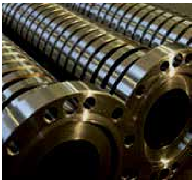
Fig. 25. Extruder screw, Cronidur 30 [ETE-11].
