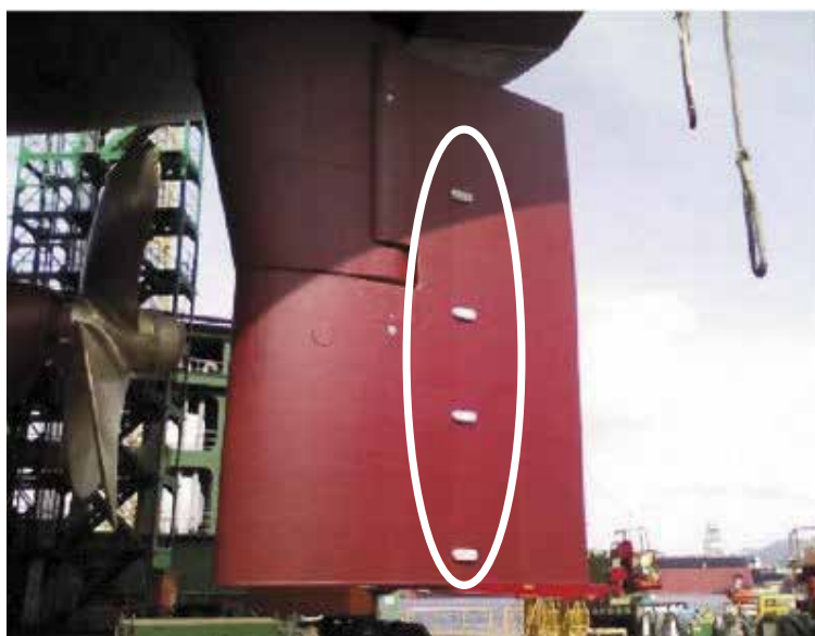
Fig. 1. Sacrificial aluminium anode attached to the hull of a ship.
