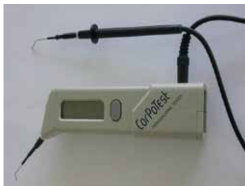
Fig. 7. Apparatus for measurement of corrosive potential.
