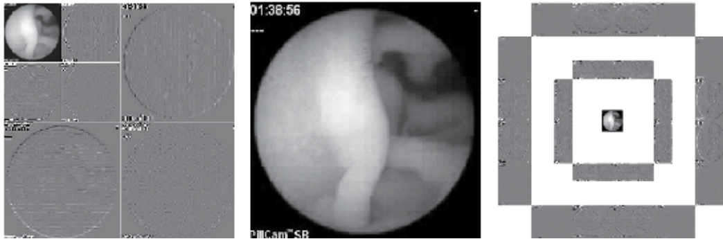
Fig. 9. Example of a capsule endoscopic frame (center) and its DWT coefficients (left) and DCT coefficients (right). Note that the number of coefficients in the DCT image is not equivalent to the other two images.
