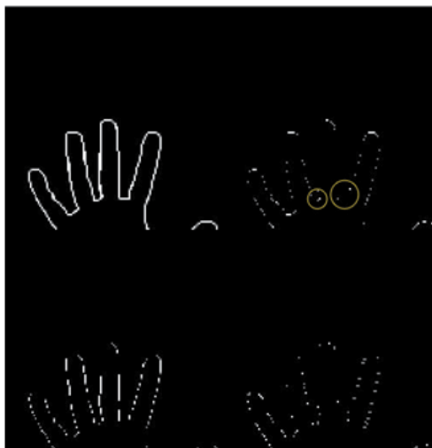
Fig. 17. A mistake in horizontal information detection in wavelet domain due to bad hand positioning.
