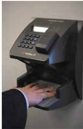
Fig. 1. Example of hand image acquisition device.
