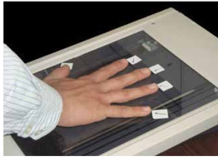
Fig. 4. Pegs on the scanner for hand positioning.
