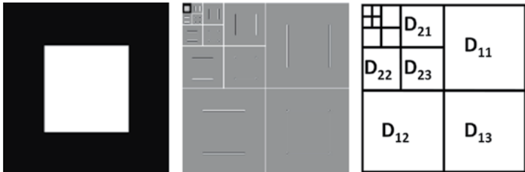
Fig. 6. Example on the directional sensitivity of the 2D Discrete Wavelet Transform (right: original image, center: DWT coefficients up to j=4 , left: correspondence between the DWT coefficients and the equations (11)-(14)).
