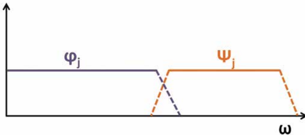
Fig. 3. Scaling function ( \phi ) and wavelet atoms ( \Psi ) spectra. Note how the scaling function ( \phi_j ) covers the spectral region spanned by the wavelet atoms until j + 1 .
