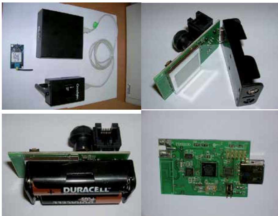
Fig. 7. Gateway based on miniPC, Mote board and base station
