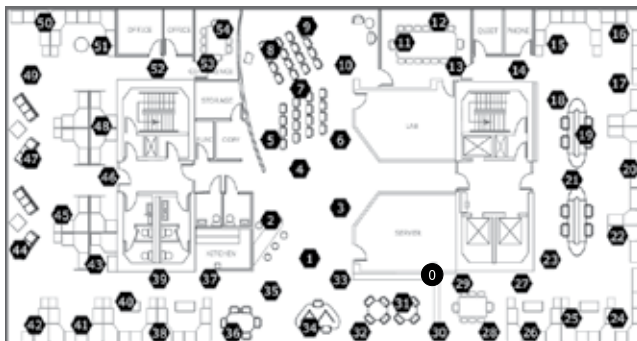
Fig. 4. Sensor nodes in the IBRL deployment. Nodes are shown in black with their corresponding node-IDs. Node 0 is the gateway node (2006, Accessed on 07/09/2006).
