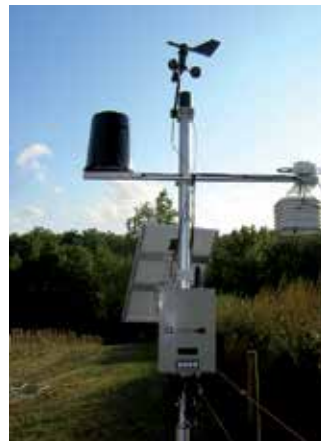
(b) VineSense GPRS Gateway with Weather Sensors
