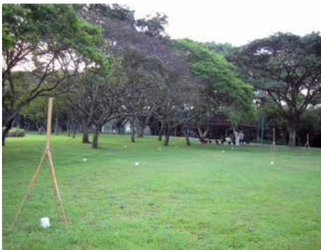
Fig. 13. ALS experiments in an obstacle ridden environment – the experiment was carried out in a 30m×30m region in a park with several trees in the region. Several of the sensors were placed behind trees, as seen in the picture.
