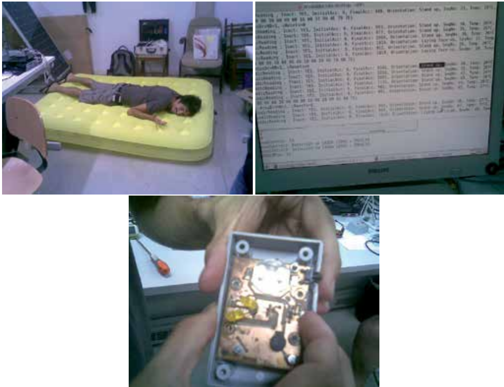
Fig. 9. Actor with accelerometer in his waist, log of data and accelerometer sensor node prototype
