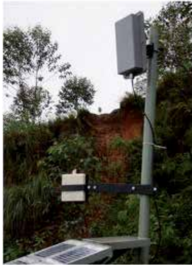
Fig. 4. Field Deployment of WINSOC Node With Miniature Antenna
