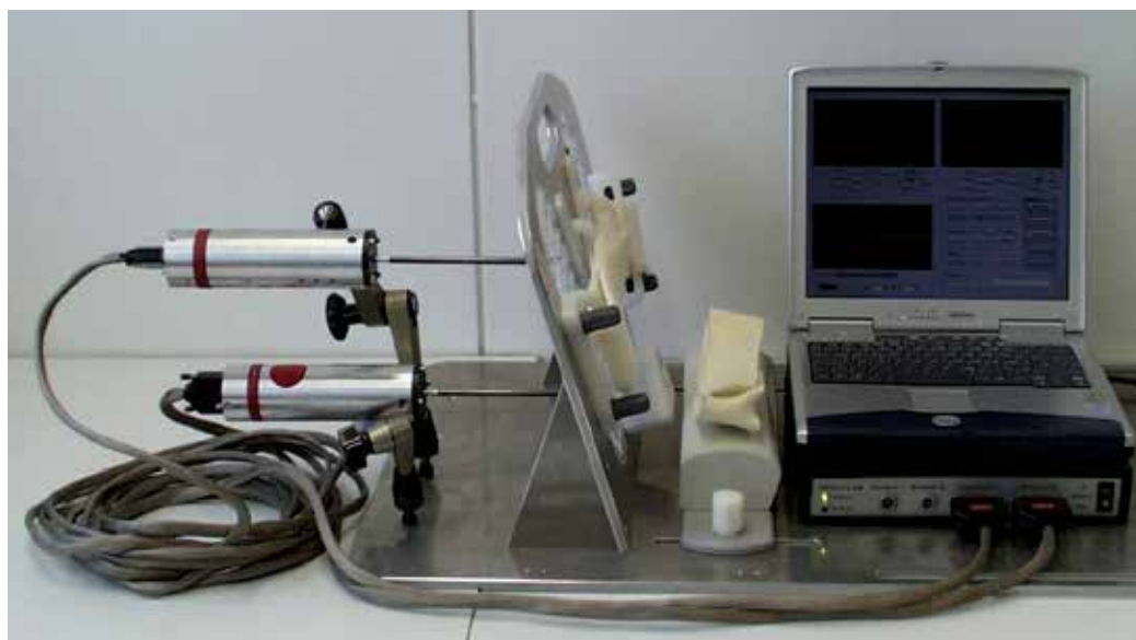
Fig. 2. Example of an electromagnetic vibrotactile stimulation system (Gallasch et al., 2006).
