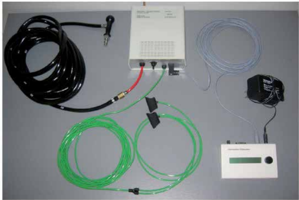
Fig. 4. Stimulator system consisting of twin finger cuff, valve box and microprocessor unit.
