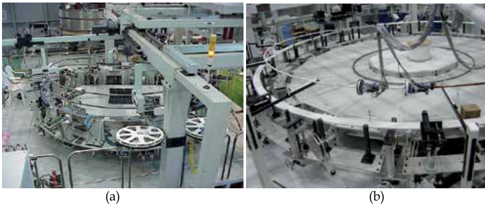
Fig. 7. The picture of coil winding stations of the TF coil (a) and PF coil (b).
