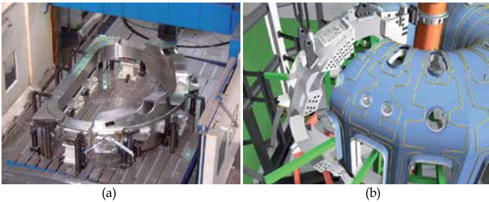
Fig. 11. TF magnet structure fabrication and assembly. Final machining after coil encasing (a) and the schematic drawing of a TF magnet installation into torus of the vacuum vessel (b).
