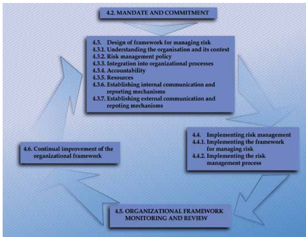
Fig. 3. Components of the framework for managing risk (Based on ISO 31000:2009)
