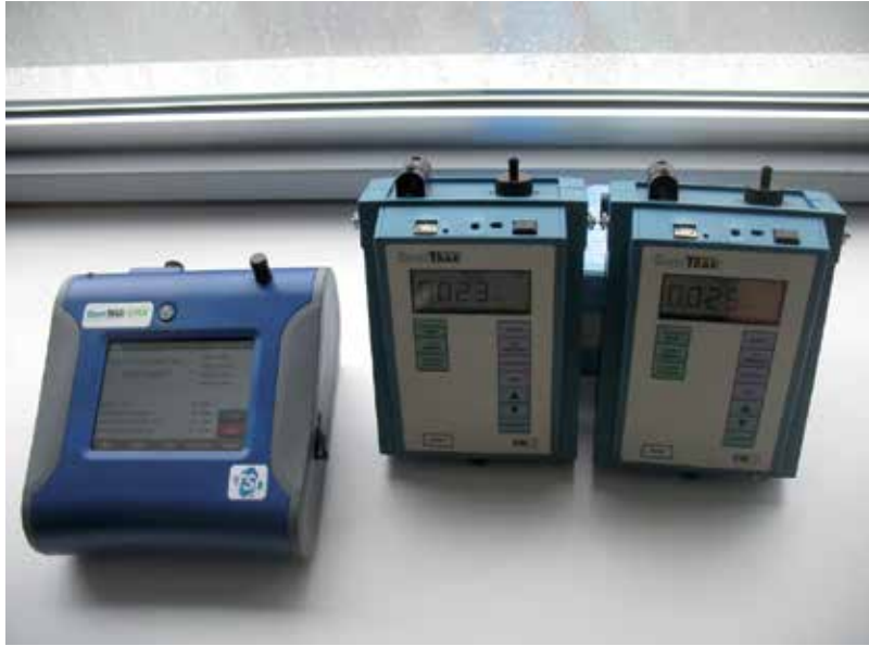
Fig. 9. PM10 devices (for example, Dust Trak model 8533/ 8520).
