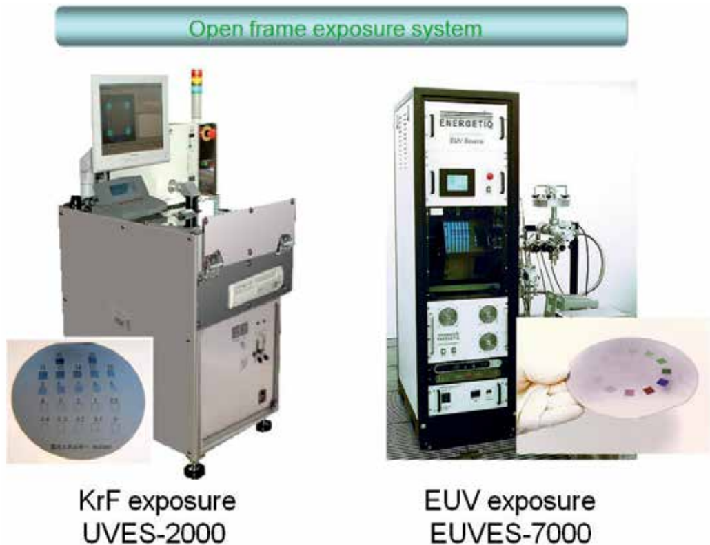
Fig. 10. Open frame exposure tool for KrF and EUV
