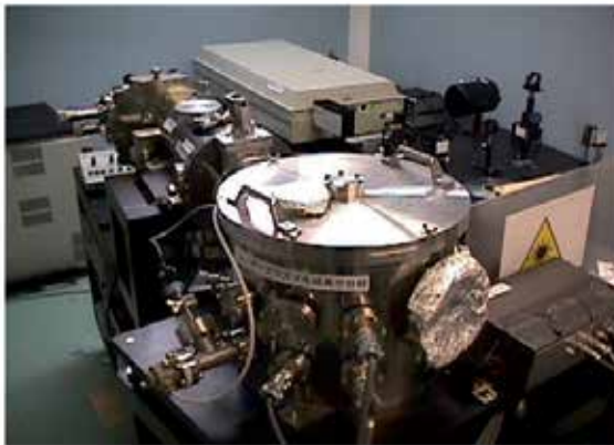
A reflectance measurement tool by laser plasma EUV light source
