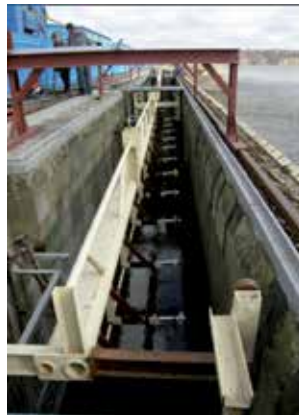
Fig. 11. Frame with fixed the current meters for traversing the hydrometric (measuring) section (author's application).
