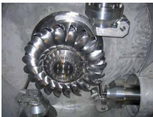
Photo 29. The Pelton runner and its 3 jets (case study La Zour).
