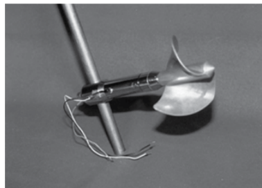
Fig. 9. Propeller-type current meter. (The local flow velocity component is measured based on the current meter rotor revolutions counted in a given time period, and the experimentally determined relationship between the current meter rotation speed and local flow velocity).
