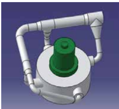
Fig. 6. 4-nozzle Pelton turbine with a progressive flow acceleration to avoid waste accumulation.
