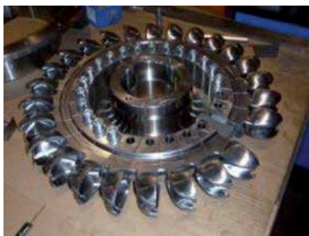
Photo 31. Achievement of a Pelton runner with mounted buckets (St Jean SHP plant, Switzerland, set in a drinking water network, H = 373 m, Q = 34 l/s, P=102 kW, 2009).
