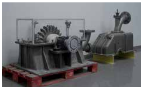
Photo 22. Tordera: a dismantled Pelton turbine.
