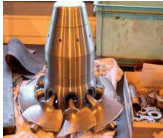
Photo 28. Kaplan runner with 8 blades during manufacturing, to be set within a drinking-water network (case study Poggio Cuculo).
