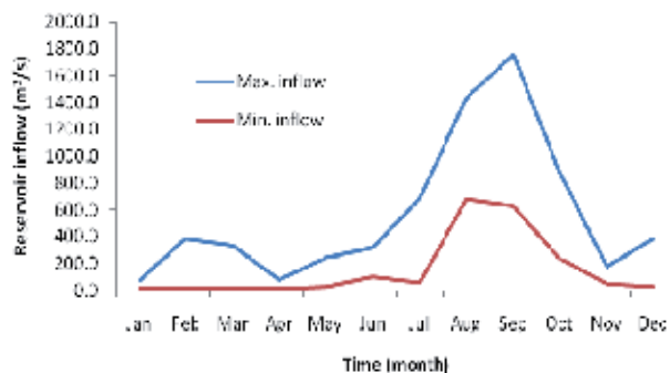
Fig. 3.7 a) Monthly variation maximum and minimum reservoir inflow at Shiroro HEP dam (1990 - 2009).
