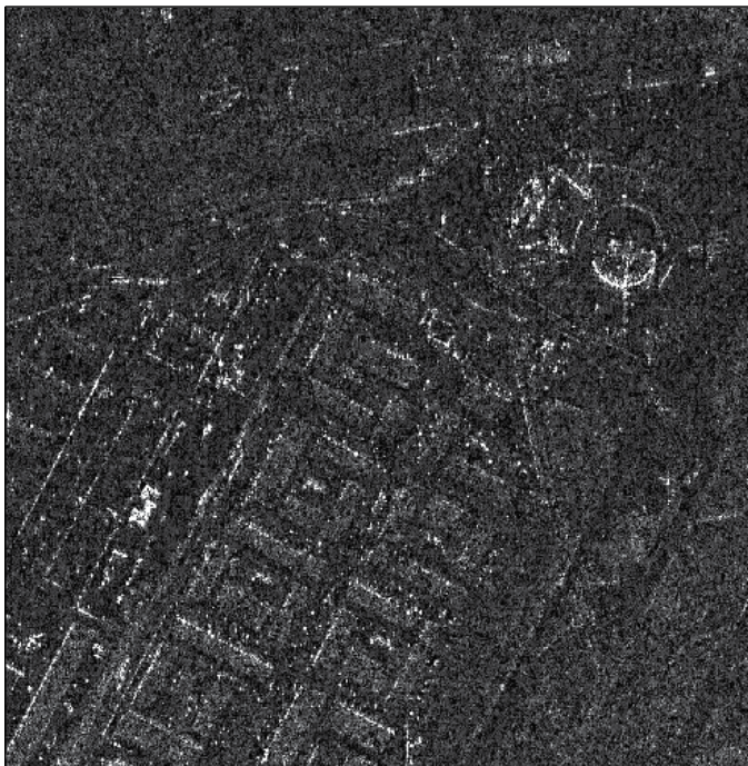
Fig. 13. SAR COSMO-SkyMed frame obtained by quantized coefficients of the overcomplete ICA basis with R=2 .
