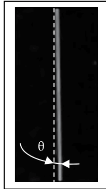
Fig. 3. Result of Sobel edge detection operator followed by thresholding and binary morphological processing (filtering) to identify the proper edge orientation ( \theta_p \sim 0.95^\circ , for \theta = 1^\circ ).
