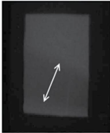
Fig. 10. Selected frame showing the indicator position and motion blur width taken from selected video sequence captured with a frame rates of 12.5 fps and for a cadmium indicator's rotation speed of 0.45 RPS.
