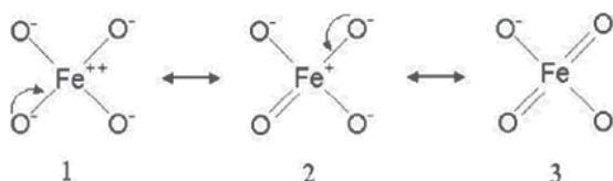
Fig. 4. Three resonance hybrid structures of Fe(VI) ion in an aqueous solution [21].
