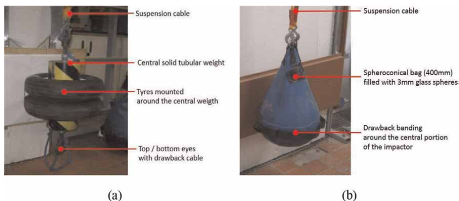
Figure 8. Conventional impactors for glass CWs: (a) twin-Tire and (b) Spheroconical bag (SB, with dimensions in mm) [61].
