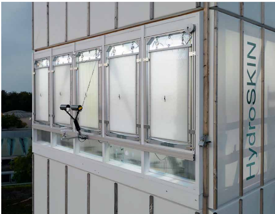
Figure 2. HydroSKIN prototypes at the D1244 experimental high-rise building in Stuttgart © S. Cichowicz.
