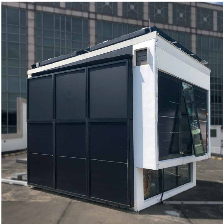
Figure 7. The mock-up of the PUBW.
