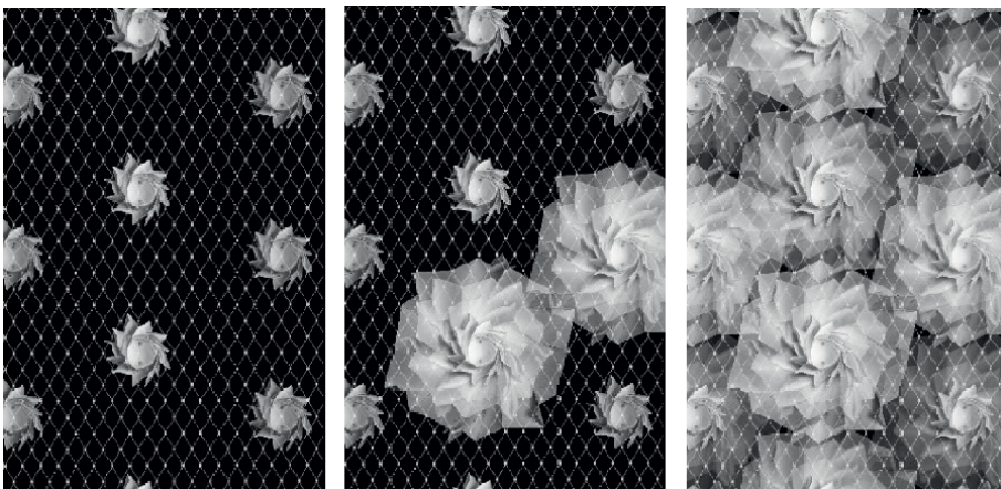
Figure 17. Visualization of PAOSS in un-activated closed state (right), targeted partial glare protection state (middle), and full-surface shading state (left) © C. Eisenbarth/ILEK.
