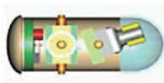
Fig. 12. IVP2 capsule steering system (taken from IVP project website)
