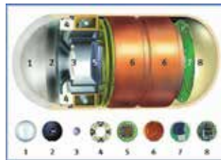
Fig. 2. The inside of the M2A capsule - 1) Optical dome, 2) Lens holder, 3) Lens, 4) LEDs, 5) CMOS imager, 6) Battery, 7) RF transmitter, 8) Antenna.
