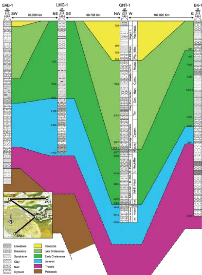
Fig. 2. Lithostratigraphic correlation of Paleozoic to Cenozoic series highlighted in the petroleum wells, showing thickness and facies variation between structures of southern Tunisia
