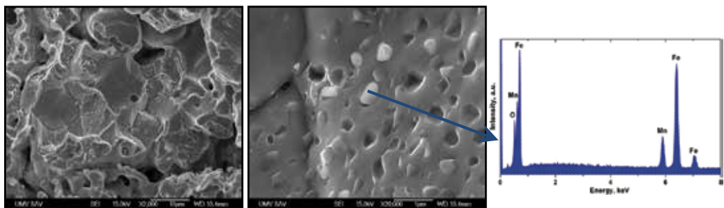
Fig. 20. SEM+EDX analysis of particulate inclusions on the inter-granular decohesion facets around ferromanganese residue after sintering at 1120°C for 30 min on the fracture surface of Fe-0.8Mn-0.5C material
