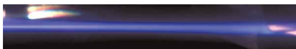
Figure 12. Photograph from above a 350 mm broad vertical argon ribbon beam of 120 mA at 3 keV. The beam at left is emerging from the third electrode of the triode. Divergence is \sim \pm 20 mrad. Scale is about 50%.
