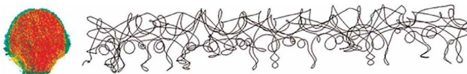
Figure 10. At left is a ray-trace of multiple electrons, viewed from the end of the arc chamber. At right is a side view of the trajectory of a single electron.
