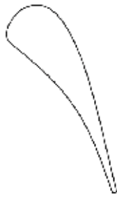
Fig. 6. Sketch and geometric data of VKI stator cascade
