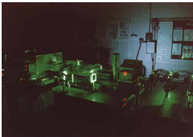
Fig. 2. Photograph of the optical arrangement for holographic interferometry at the Heat Transfer Lab of the Johns Hopkins University and the thermoacoustic refrigerator model mounted on the optical table.
