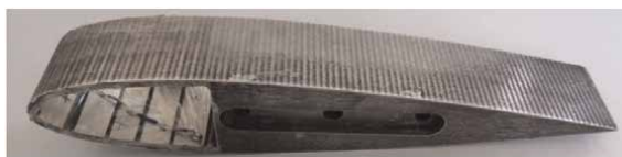
Figure 9. Test coupon of airfoil blade segment with PZT patches.
