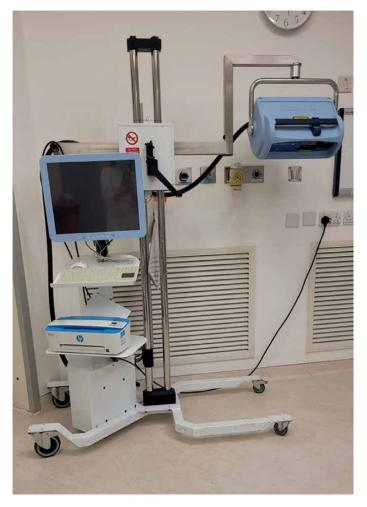
**Figure 2.** *Laser Doppler imaging device.*
