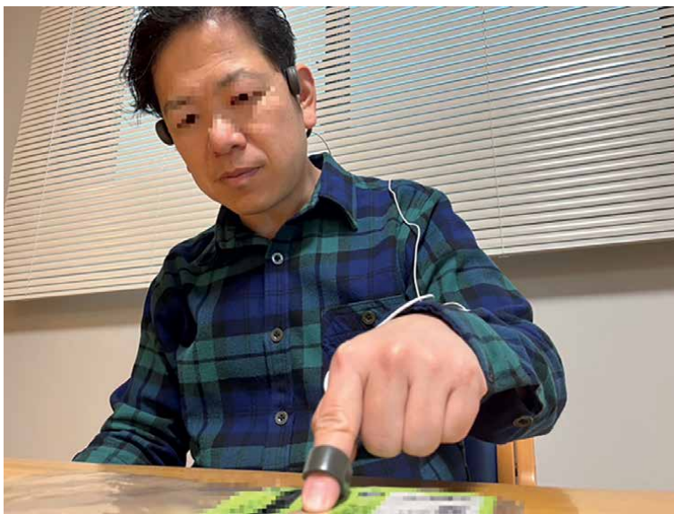
Figure 5 shows an example of a person wearing the Yubi-Recorder and performing an exercise task. A sensor attached to the left index finger senses friction information on the object, which is transmitted to a small speaker-like oscillator on the face (the mapping of the finger and face in the brain are adjacent) and fed back as compensatory deep sensory information.
