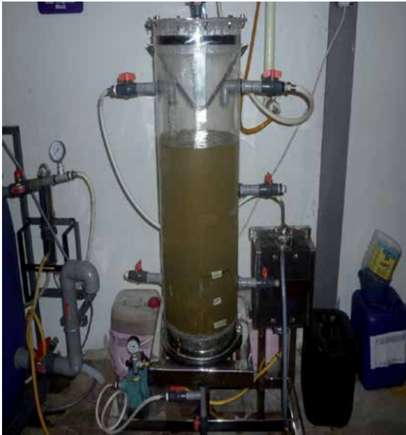
Figure 2. Schematic for Ultrasonicated membrane anaerobic system (UMAS)
