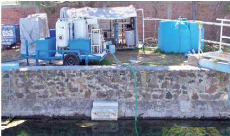
Figure 6. Pilot unit including multimedia filtration and NF.
