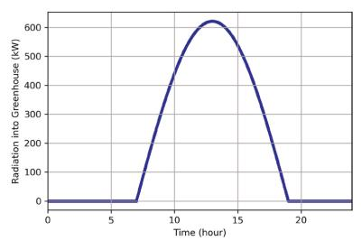
**Figure 3.** Model of the daily radiative heat load into the 1000  $m^2$  greenhouse.
