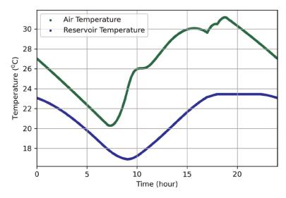
Figure 7. Greenhouse air and reservoir water temperatures over a 24-hour cycle.
