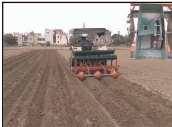
Figure 11. Maize sowing with raised bed vertical plate planter.
