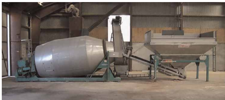
Figure 7. Dry rotary system used in small-scale fertilizer blending.
