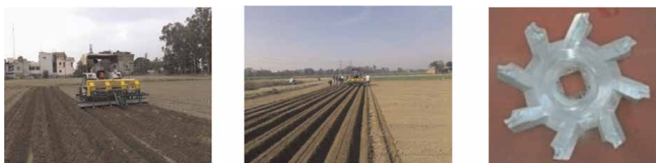
Figure 10. Maize sowing with raised bed inclined plate planter and view of metering plate.
