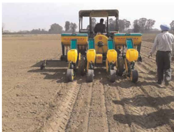
Figure 14. Maize sowing with pneumatic flat planter during 2017.
