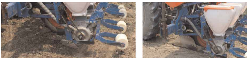
Figure 8. View of chain transmission system, press wheel and bed maker for low cost Pneumatic precision planter.
