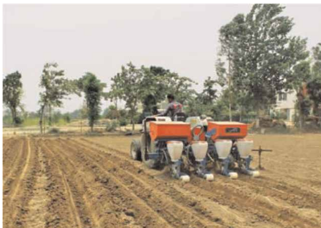
Figure 13. Maize sowing with pneumatic raised bed planter.
