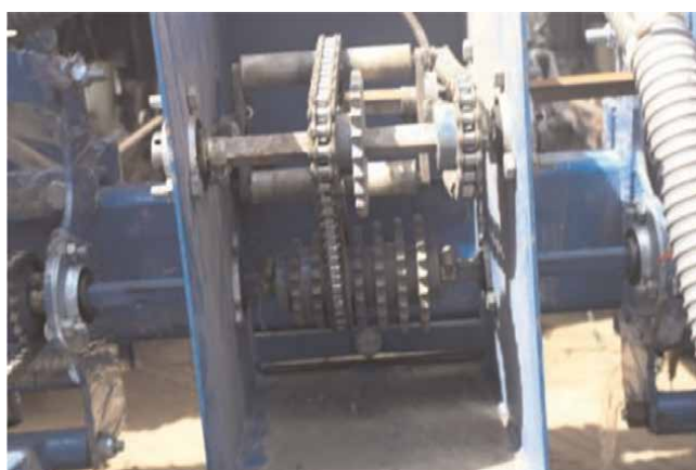
Figure 9. Chain and sprocket mechanism for varying plant to plant spacing.
