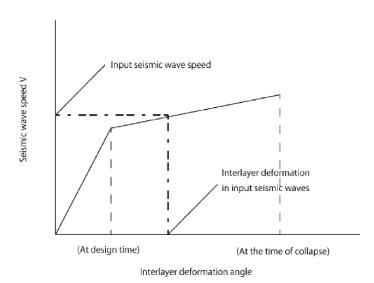
**Figure 6.** *Bilinear model at the time of PML calculation.*
