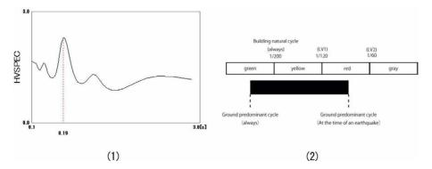
**Figure 5.** *H/V spectral ratio (1) and band determination (2).*
