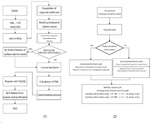
Figure 4. Overall analysis flow (1) and judgment flow (2).
