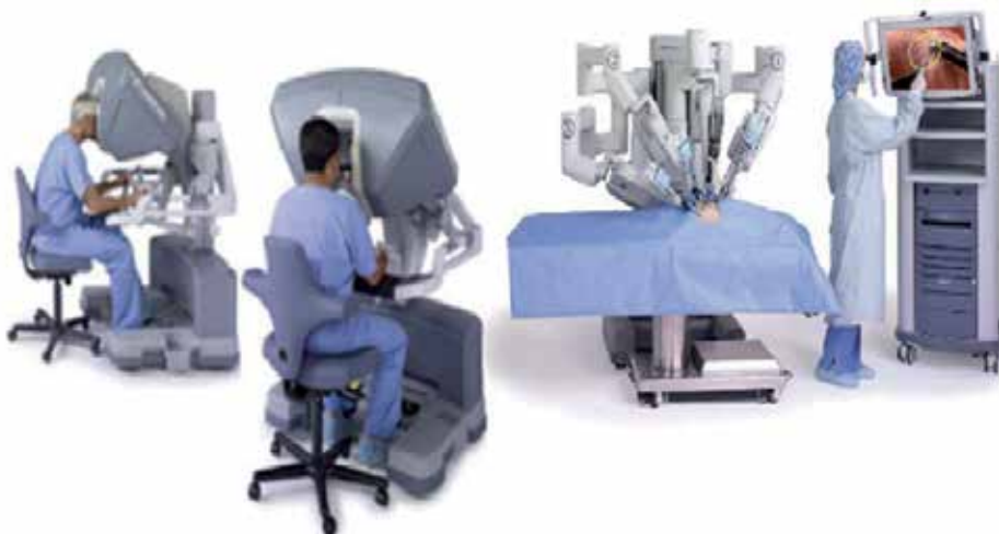
Fig. 1. Master controllers and the patient side manipulators of the new Da Vinci Si surgical system. (Photo: Intuitive Surgical Inc.)
