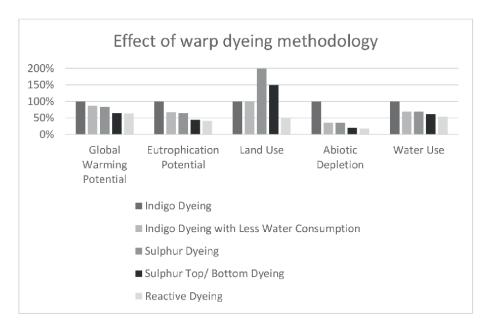
**Figure 4.** *Effect of warp dyeing methodology.*
