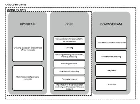
Figure 2. System boundary of the LCA study.
