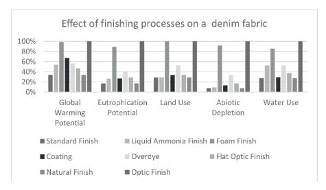
**Figure 5.** *Effect of finishing processes for a denim fabric.*
