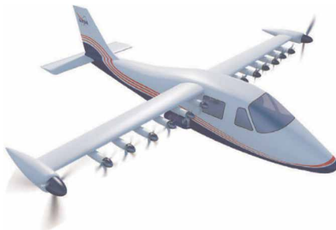
Figure 17. NASA X-57 Maxwell modification IV is testing electrical aircraft [26].
