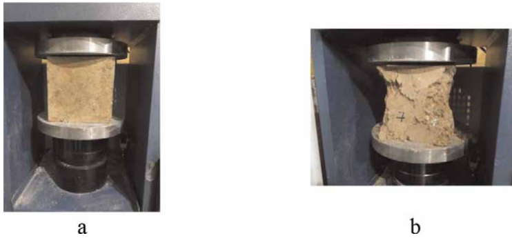
Figure 5. a) sample with 0.15 lit/m 3 additive tested in 7 days of age and b) sample with 0.21 lit/m 3 additive tested in 28 days of age.
