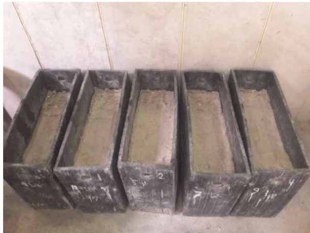
Figure 18. Ballast box samples after testing (specimens from left to right correspond to 0, 0.09, 0.15, 0.21, and 0.27 lit/m 3 of RRP 235 Special ).
