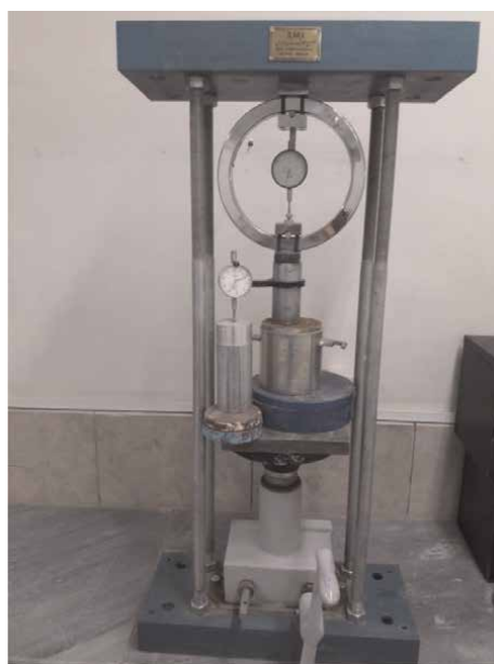
Figure 8. a) Ballast box test apparatus; b and c) ballast box dimensions; d) LVDT location [38].
