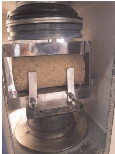
Figure 6. The sample with 0.15 lit/m 3 additive in Indirect Brazilian Tensile Test device.
