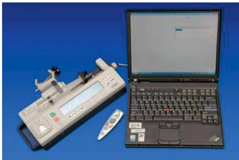
Figure 9. Computer integrated patient controlled epidural pump (first generation computer integrated infusion pump set-up using an IBM Thinkpad laptop (IBM, USA) connected to a modified syringe pump (IVAC P700, Alaris, UK).
