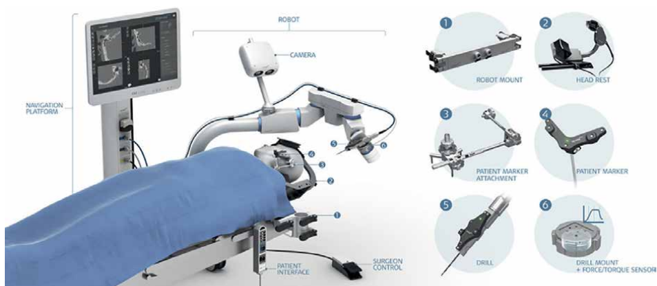
Figure 2. The HEARO® robotic system. (1) robot mount, (2) headrest, (3) patient marker attachment, (4) patient marker, (5) drill and (6) drill mount with force/torque sensor [2].
