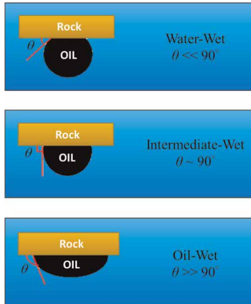
Figure 14. Schematics of contact angle for different wettability conditions of the solid-water-oil system.
