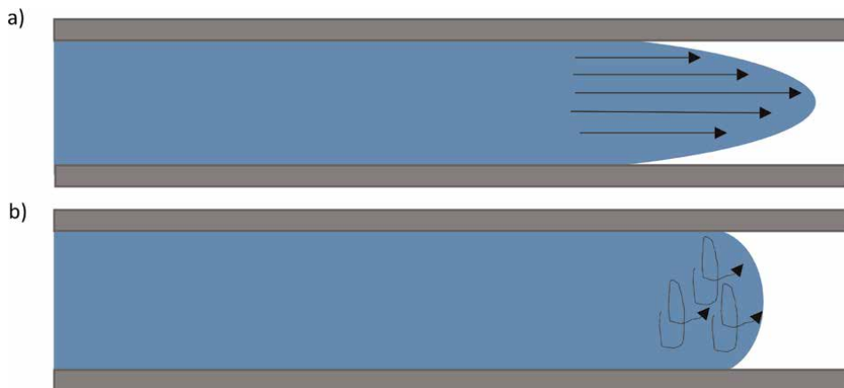
Figure 2. a) Laminar flow; b) turbulent flow.
