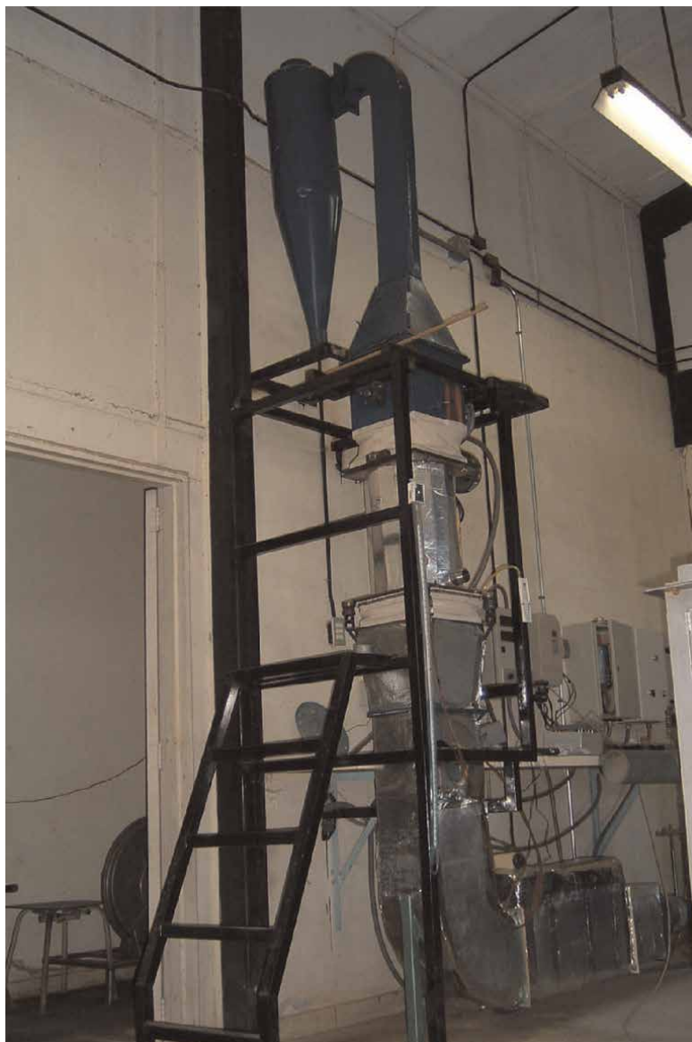
Figure 2. Overview of the fluidized bed dryer of biomass particles.
