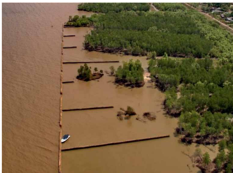
Figure 7. Wave dampening effect of bamboo T-fences, Ca Mau Province, Viet Nam (photo R. Sorgenfrei 2016).
