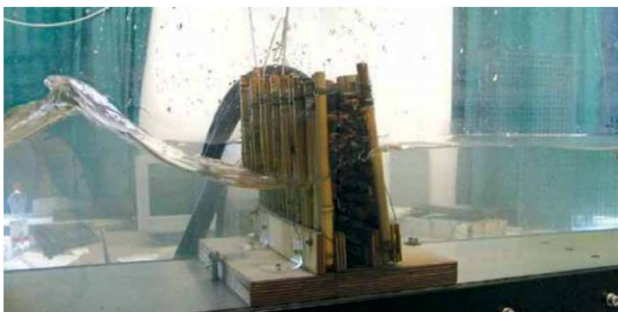
Figure 4. Physical modelling of wave transmission through bamboo fence, scale 1:20 (photo T. Albers 2010).
