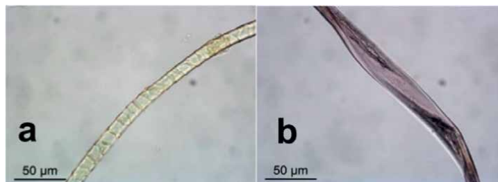
Figure 5. Optical microscopy image of merino loose wool (a) and cotton fibers (b) obtained in transmission mode. (500 X).
