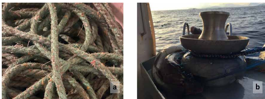
Figure 2. Worn-out lead line (a) and a typical gillnet hauler (b). Photo: SINTEF.
