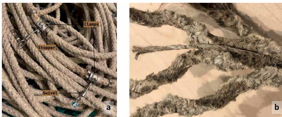
Figure 4. Autoline with stoppers, swivels, and clamps (a) and a worn-out autoline with the cords split apart (b). Photo: SINTEF.
