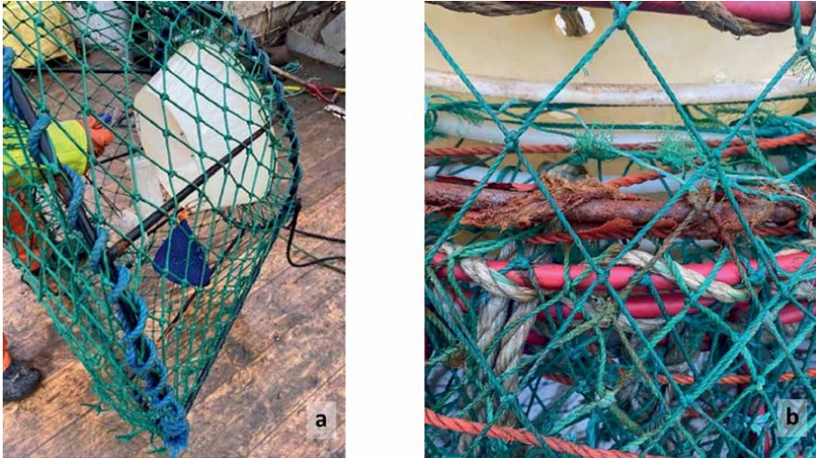
Figure 3. Snow crab pot (a), with cracked coating (b). Photo: SINTEF.
