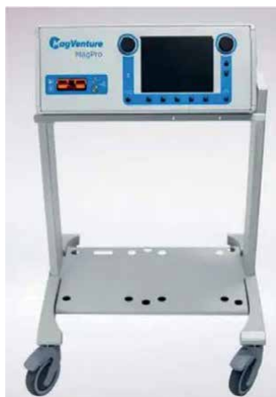
Figure 2. Example of a transcranial magnetic stimulator [11].
