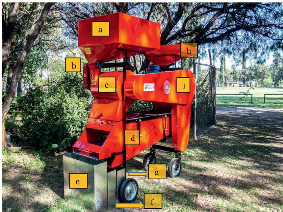
Figure 4. Components of the “algarrobo” threshing machine (Cosiansi, 1991): a) pods hopper, b) shredder, c) threshing cylinder I, d) sieves, e) flour tray, f) knuckles tray, g) seed tray, h) hopper for knuckles, i) threshing cylinder II.
