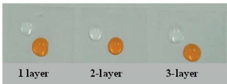
Figure 13. Contact angle of a drop of chitosan (orange) and PSS (clear) on different chitosan/PSS coating layers.
