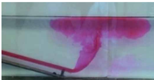
Figure 8. View of an experiment carried out in the fluid mechanics' laboratory of the physics department, Las Palmas university, gran Canaria. It is a scale model of an underwater outlet discharge. An experiment was conducted to determine the distribution of effluent with a lower density than the receiving medium and thus calibrate a numerical model of contaminant distribution (video 1).
