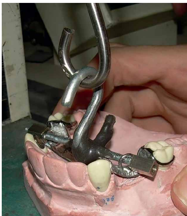
Figure 5. Pulling device installed on the metal bases for testing.
