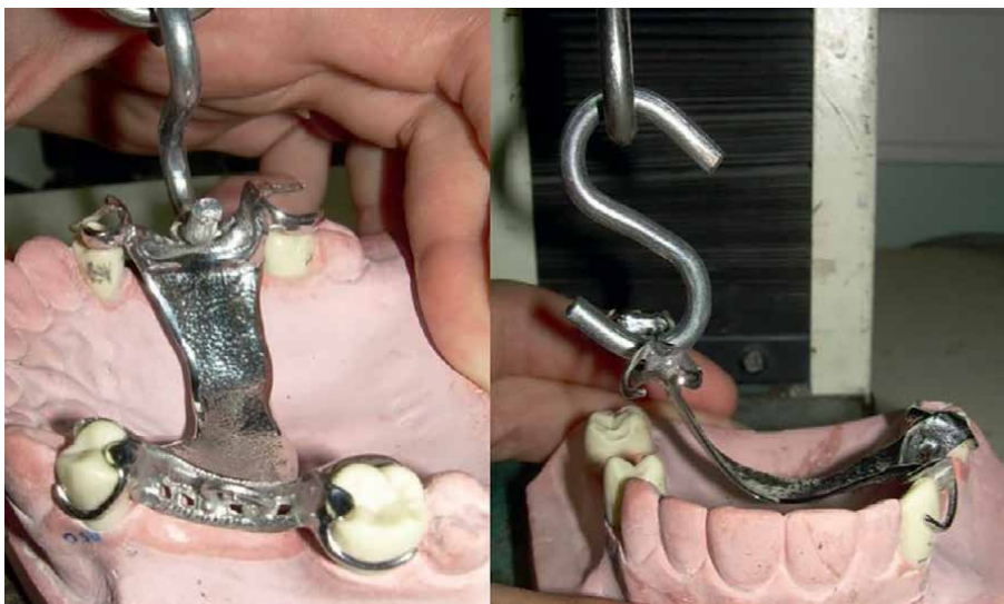
Figure 6. Pulling device installed on the metal bases for test execution.
