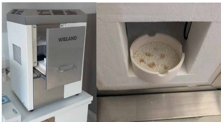
Figure 11. Sintering zirconia frameworks.
