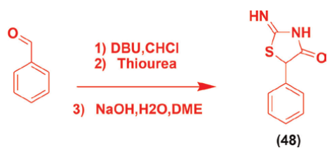
Figure 15. Synthesis of thiazolidinone by Jieping et al.
