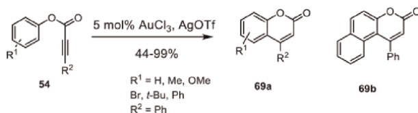
Figure 37. Method for preparation of coumarins catalyzed by \text{AuCl}_3 .
