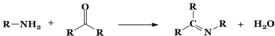
Figure 6. Synthesis of SB by condensation reaction.
