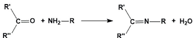
Figure 1. General scheme of formation of Schiff bases.
