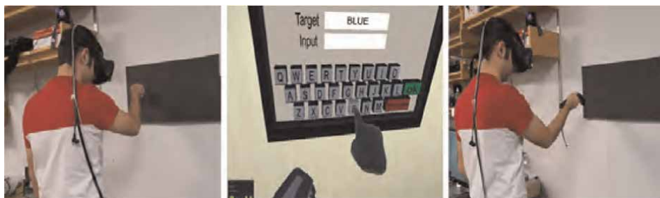
Figure 1. An example of a prototype virtual keyboard system using a foam board as a haptic proxy [20].
