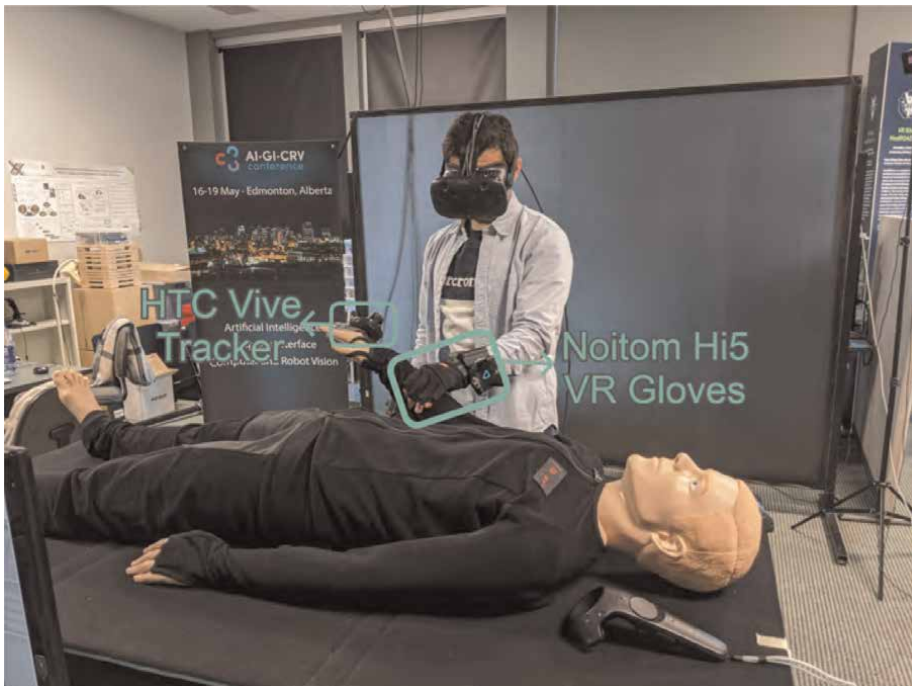
Figure 3. Proxy haptic system composed of a tracked mannequin tracked using HTC Vive beacons and a syringe tracked by a wand.
