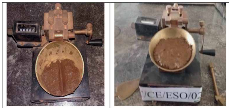
Figure 4. Liquid limit test instrument for measurement.
