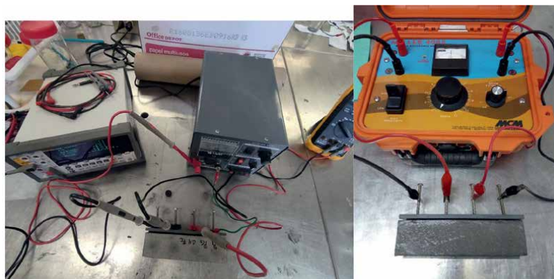
Figure 5. Experimental arrangement for determination of EC electrical conductivity.
