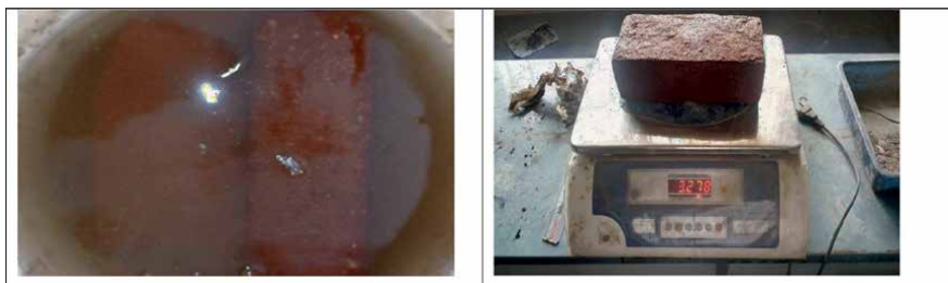
Figure 9. Sawdust bricks during water absorption test.
