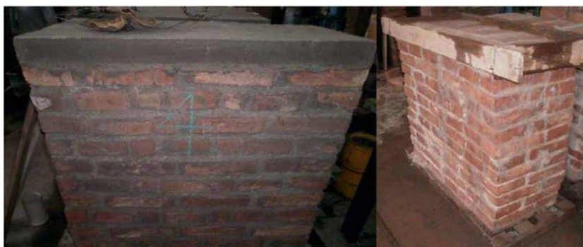
Figure 7. Preparation of masonry specimens [33].
