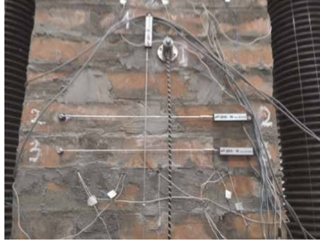
Figure 7. Placement of strain gauges on the sample surface.
