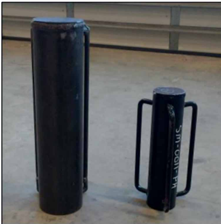
Figure 18. A comparison of the Horn 2" tube well installation drive sleeve (left) and the Shaver (Graettinger, Iowa) steel fence post driving sleeve [10].
