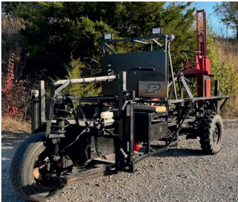
Figure 16. Well-Driver PUP vehicle in operational configuration with the hydraulic driving ram erected [37].
