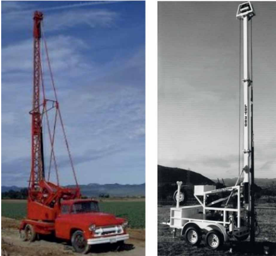
Figure 4. Truck-mounted cable tool rig (left) and trailer-mounted tool rig (right) [31].
