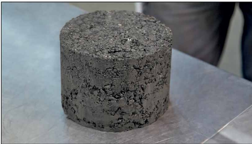
Figure 5. Pill. Core from foamed bitumen stabilized asphalt layer [44].
