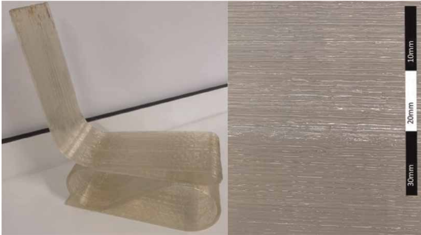
Figure 9. Closeup of single-cycled design showing test part (left) and regular layering (right). Scale bar shows a mark every 10 mm.
