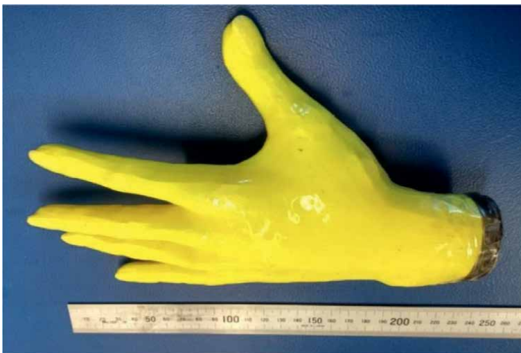
Figure 2. Example of a ‘hand surrogate’ shell additively manufactured in ABS for the heat loss assessment of the gloves.
