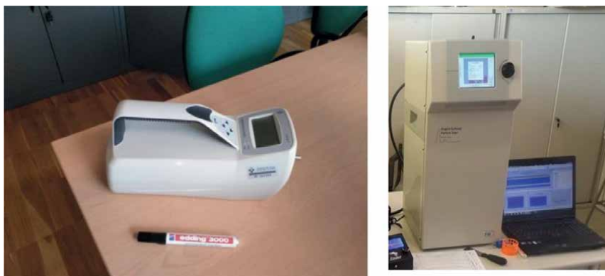
Figure 3. Nanoparticles sampling devices: CPC 3007 (left) and EEPS3090 (right).
