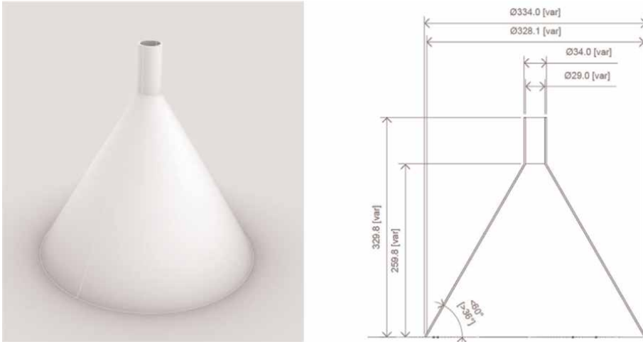
Figure 4. Test parts (II). Hopper showing dimensioning constraints.
