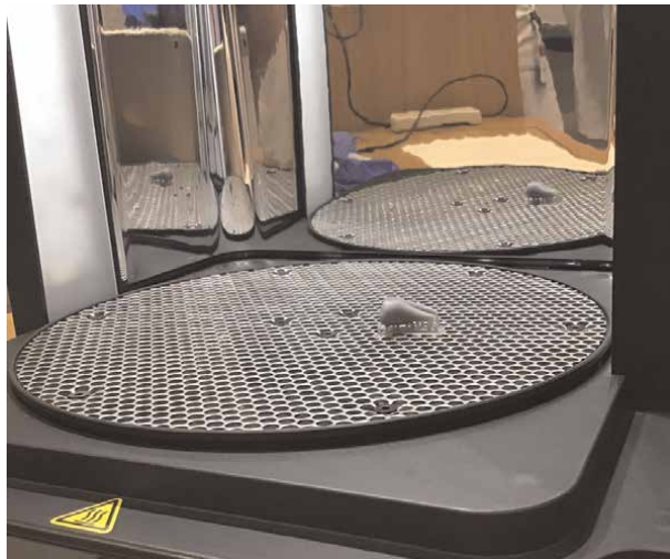
Figure 4. Already printed molar tooth, after using form washer, on the platform of form cure.
