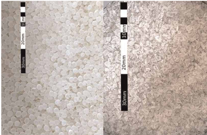
Figure 11. Photography of \phi 2– \phi 4 mm PLA spherical and \phi 1.5– \phi 3 mm flake-shaped pellets used in the experiment.
