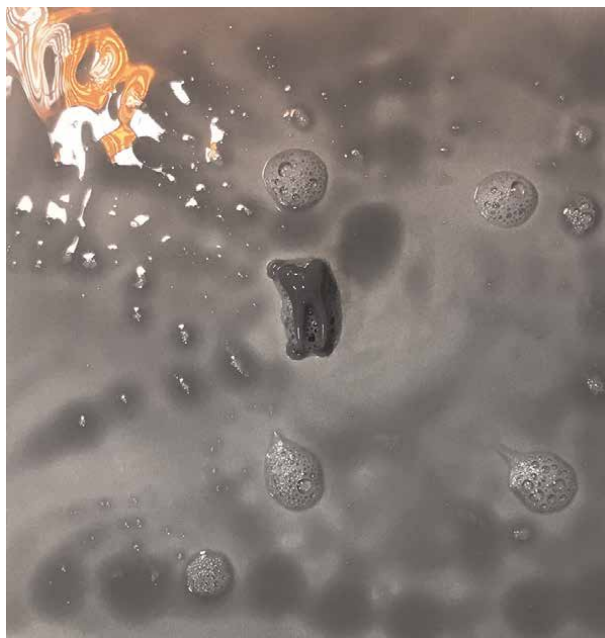
Figure 3. Printed molar tooth on the platform, before inserting into the washer. Tooth length is 18,08 mm.
