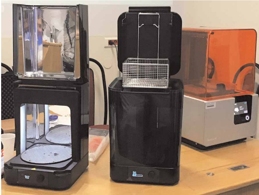
Figure 1. 3D printer kit (Formlabs), from left to right: Form cure, form wash and 3D printer.
