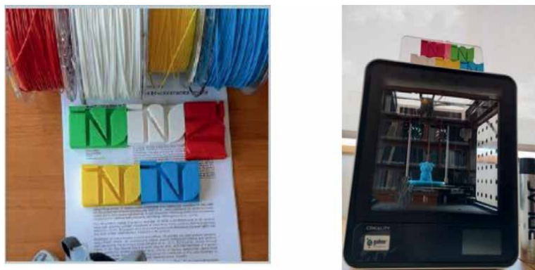
Figure 4. Different 3D printing filaments (left) and 3D printer (right).
